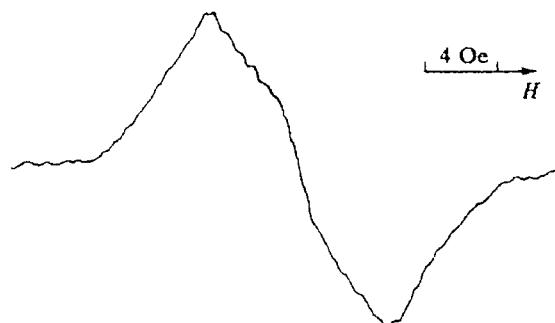
Fig. 1. ESR spectra of the polymer 1—aniline—cyclohexanone system 1 h after mixing of the components.
